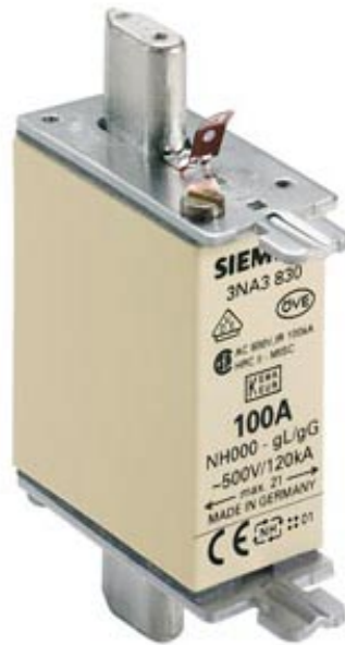
LV HRC FUSE LINK GL/GG WITH NON-INSULATED GRIP LUGS WITH FRONT INDICATOR SIZE 000, 100A, AC 500V/DC 250V
