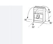
With residual-current release XFI: - NZM1, N1, NZM2, N2: vertical and 90° in all directions 90° in all directions
