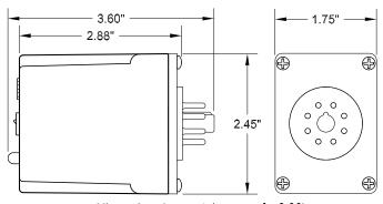
(dimensions have a tolerance of ± 0.06) Shows No Power Applied
