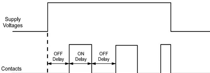
When the supply voltage is applied, the OFF cycle begins timing. Upon completion of the delay, the internal relay energizes and the ON cycle begins timing. The timer will continue cycling until the supply voltage is removed. ON and OFF cycles can be of equal or unequal durations.
