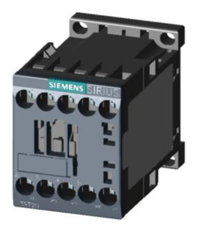
CONTACTOR, 3AC, 5.5KW/400V, 1NO, AC400V, 50HZ, 400...440V 60HZ 3-POLE, SZ S00 SCREW TERMINAL
