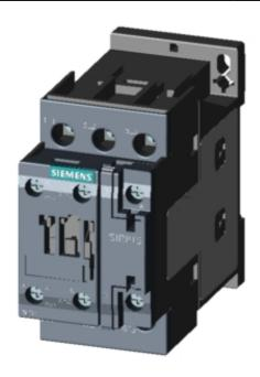
CONTACTOR, AC-3, 11KW/400V, 1NO+1NC, AC 220V 50/60HZ, 3-POLE, SZ SO SCREW TERMINAL
