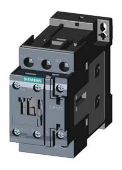
CONTACTOR, AC-3, 15KW/400V, 1NO+1NC, DC 24V, 3-POLE, SZ SO SCREW TERMINAL
