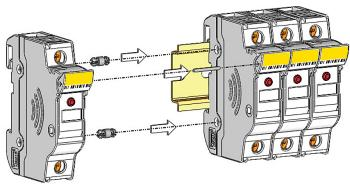
Gang multiple poles to meet application requirements using kit catalog number JV-L (gangs up to four poles).
