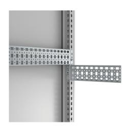
**Descripción:** Universal profile for both depth and width fitting on the 25 mm DIN hole pattern of the enclosure's frame or in combination with the CLPF and VB profiles. The 75 mm wide profile is equipped with three rows of holes of which one is turned 90°. This makes it possible to mount the CLPF profiles in both directions. The CLPK can be secured by the use of self tapping screws.
