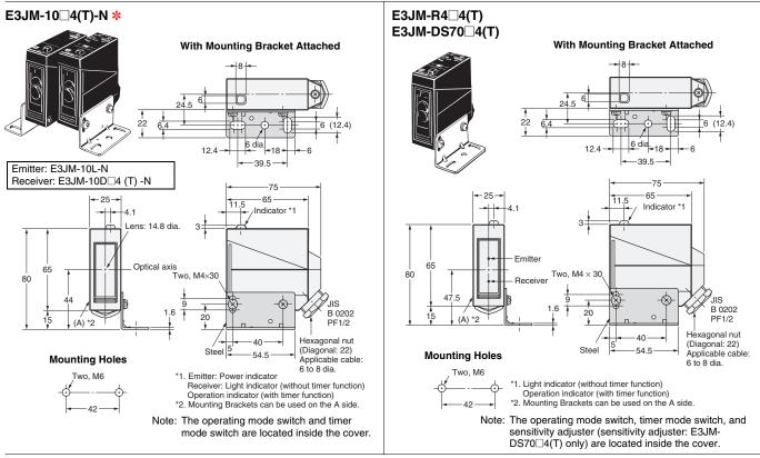
\* Models numbers for Through-beam Sensors (E3JM-10□4(T)-N) are for sets that include both the Emitter and Receiver.
