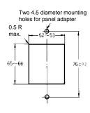
Note: recommended panel thickness is 1 to 3.2 mm..
