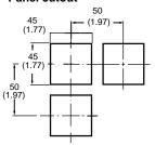
Note: Recommended panel thickness is 1 to 3.2 mm.
