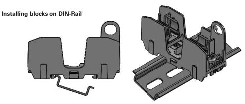
Place one edge of DIN-Rail in fuse block base, then rotate block down until it clicks into place.
