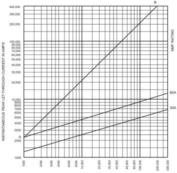
RMS SYMMETRICAL CURRENT IN AMPS A-B = ASYMMETRICAL AVAILABLE PEAK (2.3 X SYM RMS AMPS)
