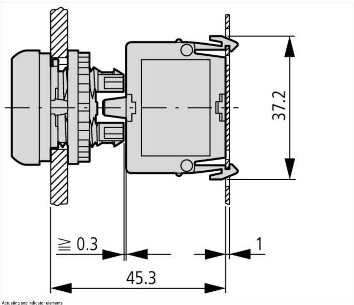
Actuating and indicator elements Base fixing
