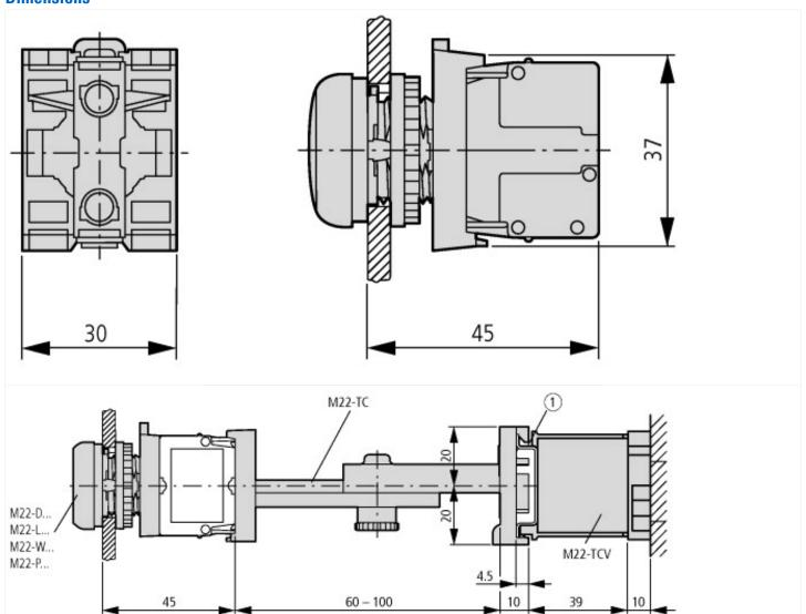
Pushbuttons and indicator lights with M22-TC telescopic clip and M22-TCV extension
