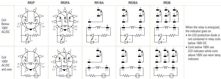
LED indicator while coils above 100V use neon lamp Signaling Lights
