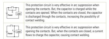
Generally, switching a DC inductive load is more difficult than switching a DC resistive load. Using an appropriate arc suppressor, however, will improve the switching characteristics of a DC inductive load.
