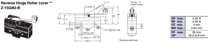
\*\* The pin plungers of reverse-type models are continuously pressed by the actuator levers with compression coil springs and the pin plungers are freed by operating the levers. Reverse-type models are highly vibration- and shock-resistive because the pin plungers are normally pressed. Note: Unless otherwise specified, a tolerance of ±0.4 mm applies to all dimensions.
